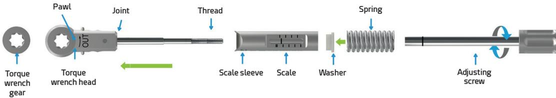
**NOTE:** the individual components come apart when the screw is removed. To assemble the torque wrench, simply assemble the individual parts in the same order and tighten the adjusting screw.
