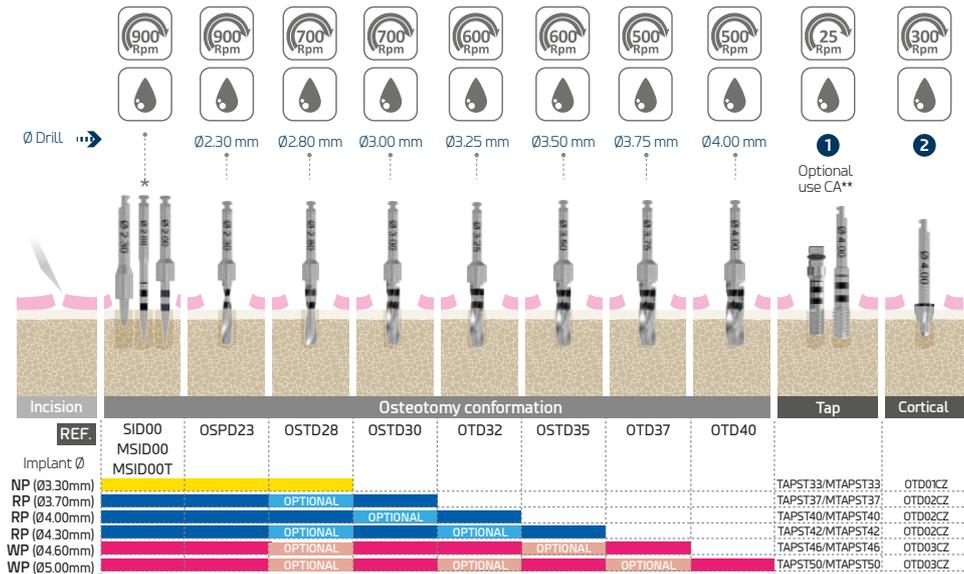
\* When drilling Type I/Type II bone, increase the speeds indicated above by 200 rpm. Use mm-graduated lance drill MSID00/MSID00T before using the pilot drill.
