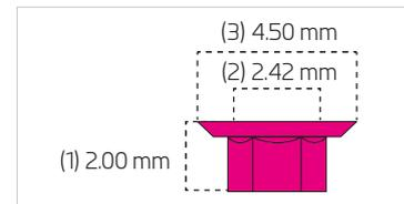
(1) Internal hex depth. (2) Distance between faces of the internal hex. (3) Diameter of working platform.
